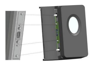
5. The side-attach peripheral connection cover is now removed as seen.
