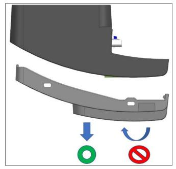
2. Gently remove the side cover by prying the 2 ends outwards (see arrows) with a small screwdriver.
