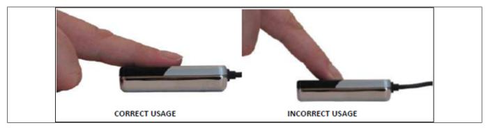
To encourage flat finger placement, it is important that the tilt angle of the module's window be horizontal or even slanted forward (away from the user) in all applications where the module is one foot or more below eye level.
