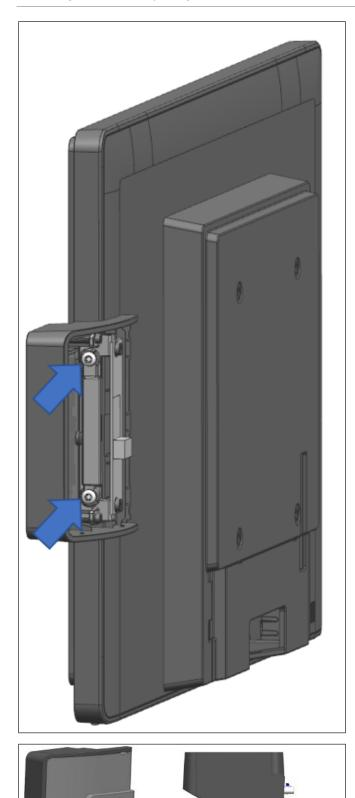
9. Then put on and tighten two M3x7 screws with Torx screwdriver (T-10).
